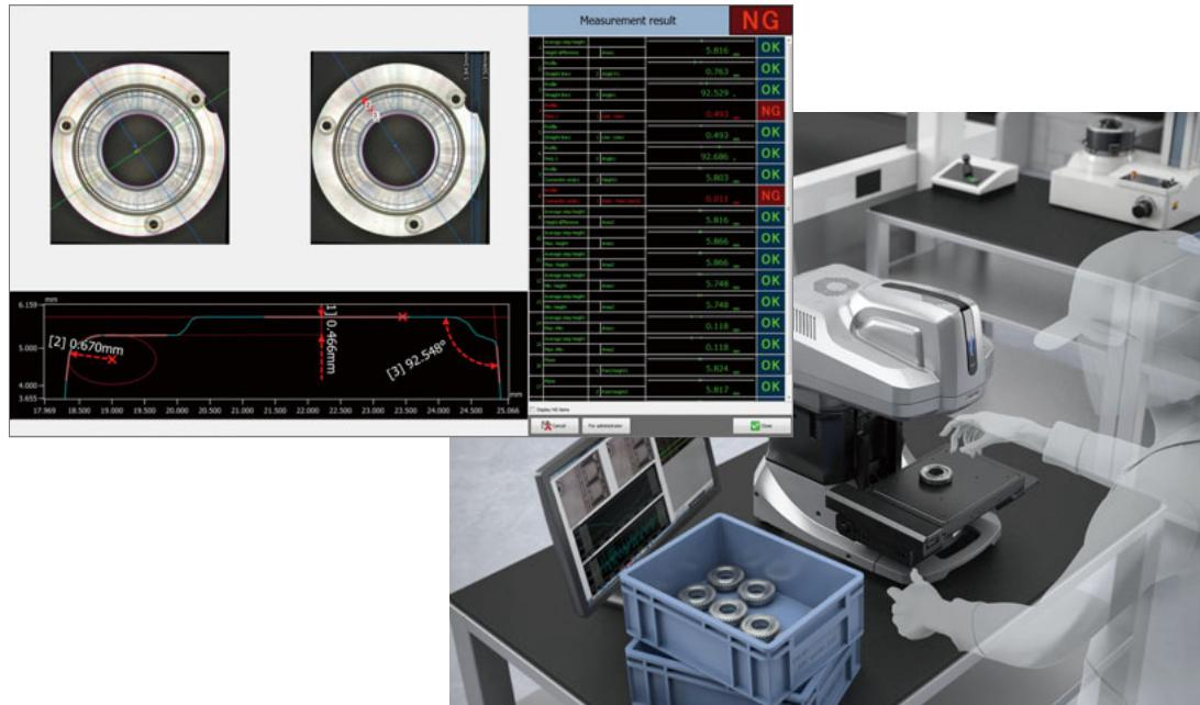
Based on registered tolerances, pass/fail (OK/NG) judgment can be made as soon as measurements are taken. This saves inspection time in various quality and analysis applications such as setting prototype conditions or performing acceptance inspections.
