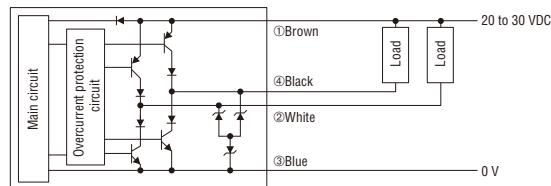
When I/O wire (④ black) is set to Input (external input)
