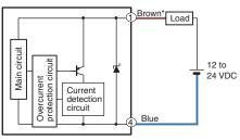
Load can also be connected between blue wire and negative terminal of power supply The M8 sensor does not contain short-circuit protection or a current detection circuit 1 and 4 in the circuit diagram shows the pin number of the connector type
