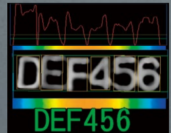
Height-extracted image (Free-form plane) + OCR
