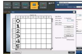
Connecting to the CV-X automatically develops OCR for use with the MK-U. No bothersome dictionary registration is required.
