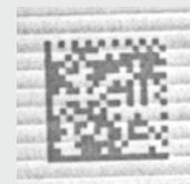
Codes marked on milled surfaces
