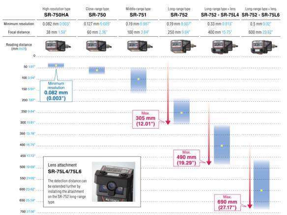
The reading range above is a value measured with a KEYENCE test label. Max. 305 mm 12.01\*, 490 mm 19.29\*, and 690 mm 27.17\* are for DataMatrix (cell size 0.5 mm 0.02\*).
