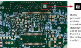
processina immediate detection of 2D codes even if there is a codelike pattern in the field of view.
