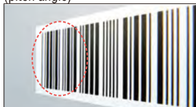
Problem: Drop in received beam intensity, bar ratio variations
