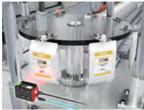
Error-proofing product types in filling machines
