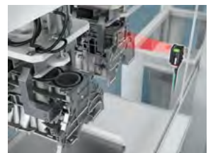
Reading engine parts during conveyance on a gantry loader
