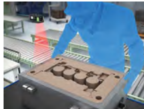
Error-proofing patterns for sand mold casting
