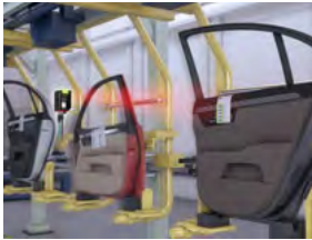
Reading instructions during hanger conveyance
