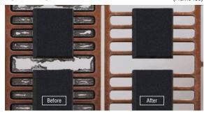
Burrs can be removed with high precision and without damaging the frames.
