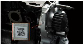
2D codes are marked at high speeds even on casted surfaces. This makes quality improvements and reductions in marking time possible.
