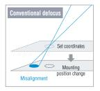
Because the mounting position is physically shifted, the irradiation position and character size are also misaligned in relation to their settings.
