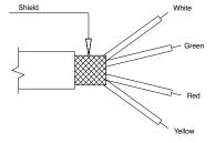
\* The screen is isolated from the transducer body. It is recommended that the ground is connected at the instrument end.
