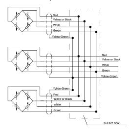
In systems that use several cells, the parallel connection automatically sums the loads on each individual cell.
