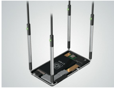
Smartphone chassis flatness inspection
