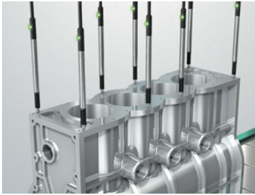
Flatness measurement of engine block
