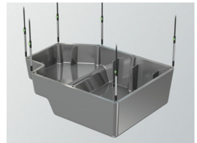
Oil pan flatness measurement
