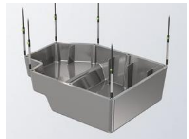
Oil pan flatness measurement
