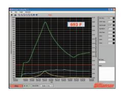
ProView PC software is compatible with Williamson Pro Series sensors. It may be used to log and analyze data and to make remote sensor adjustments.
