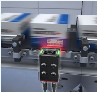
Reading barcodes off individual moving packages on a cartoning machine
